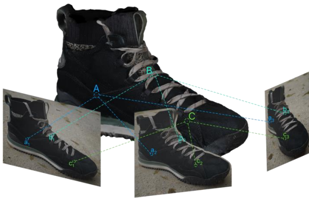
FIG. 1. Obtaining the key points of the object from images I_1 , I_2 , and I_3 taken by cameras P_1 , P_2 , and P_3 .
