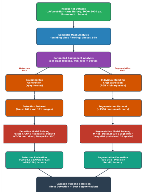
FIG. 4. Proposed end-to-end methodology pipeline for building damage assessment from RescueNet dataset through preprocessing to model evaluation and cascade selection.
