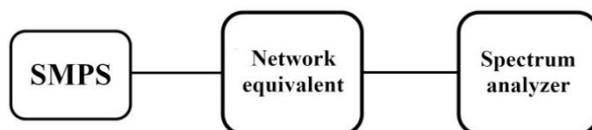
**FIG. 6.** Circuit diagram of the SMPS transformer-induced noise measurement setup.
