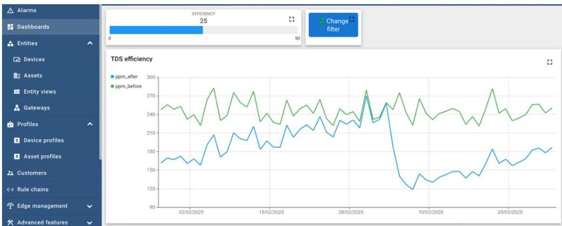
FIG. 5. Water quality monitoring interface on the ThingsBoard platform.
