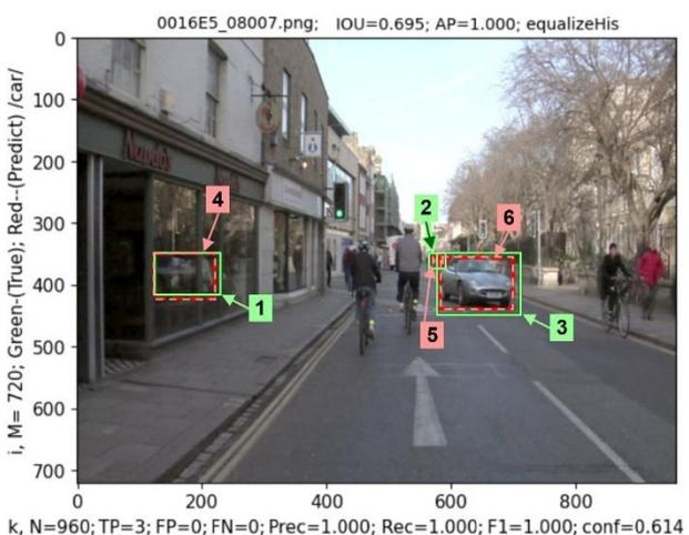
FIG. 3. Vehicle detection on the image after histogram equalization.
